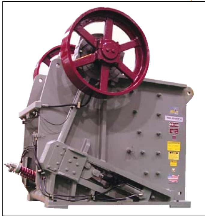
The model 4448 Iron Giant Jaw has a longer crushing chamber and shallow nip angles.
