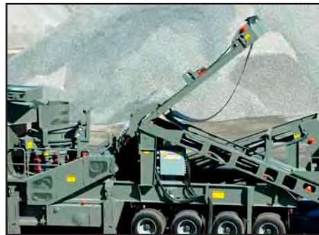
The feed conveyor folds to allow access to the cone for maintenance.
